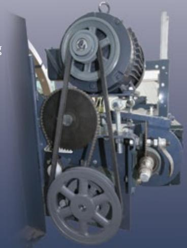
**H.** Optional—the individual grease lines assure positive lubrication from the zerks on the door frame to the worm gear drive assembly.
