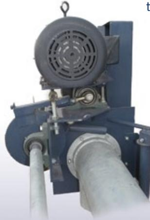
**E.** A hefty 1 ¼ inch diameter, the shaft holding the discharge hatch in place is stronger for a tighter, snugger fit. With less chance of hatch misalignment, the 8900H can better preserve and protect the ensiled feed.
