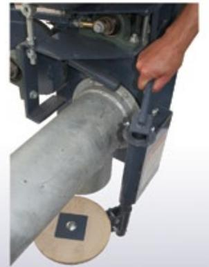
**F.** A spring-loaded ratchet drive will stop the sweep auger advancement if the sweep arm encounters an obstruction or difficult material. This provides overload protection. Before the arm advances, the sweep auger can work on the obstruction or material.
