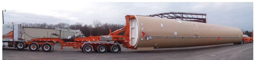
The longest factory-welded tank load transported over the road – 186' long, 185,000 lbs.
