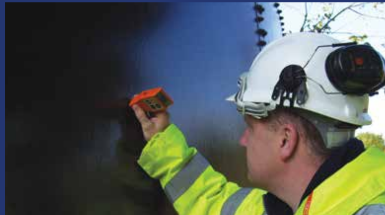
Undertaking a UTM inspection
