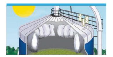
When the gases cool in a Harvestore structure, pressure decreases. The inward vacuum-like force pulls on the breather bags and (like inhaling) they inflate. The air in a properly maintained breather bag does not contact the feed. This greatly lessens the dilution of valuable fermentation gases and contributes to a beneficial fermentation environment. There is no equivalent accessory capable of performing this function in a conventional top-unloading silo, bunker or trench.
