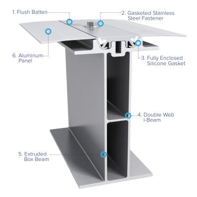
The flush batten OptiDome® is a next generation geodesic dome from CST. Combining premium features and incorporating the engineering experience and heritage of Temcor and Conservatek®, OptiDome sets a new standard in engineered aluminum cover technology.
