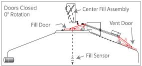
Push-Button Fill Doors are simple to use - just push a button on the convenient ground level control panel. A touch of the OPEN DOORS button opens the center fill and vent door and positions the Model 135 cent fill chute for filling. A series of indicator lights are illuminated to show doors are open, closed, in motion, or when structure is full.
