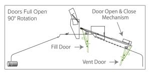
Push-Button Fill Doors™ are a convenient option for Harvestore Systems. The Push-Button Fill Door system replaces the need for climbing to the top of a Harvestore structure and manually opening and closing the center fill and air exhaust door for normal fill operation.
